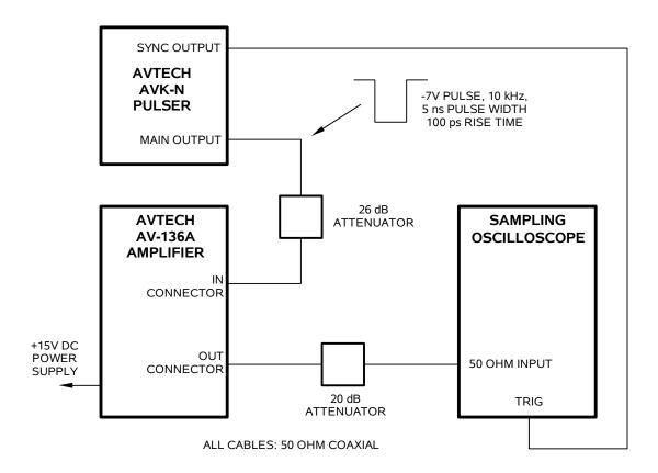
The factory test set-up is shown above.
